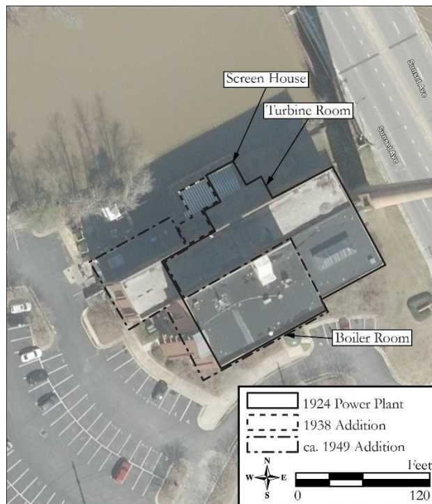
Figure 2. Evolution of the Rocky Mount Power Plant building (NC OneMap 2024).
